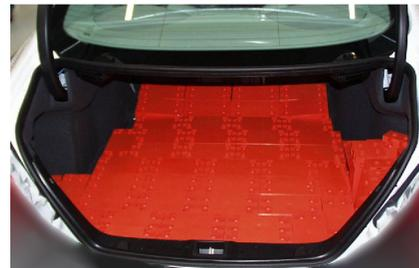
Figure 1: Physical measurement according to DIN 70020
